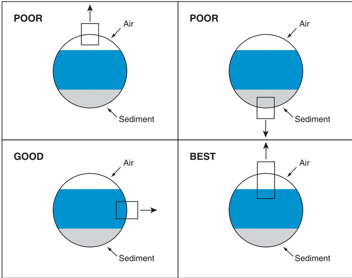
FIGURE 5 (Installation Example)
